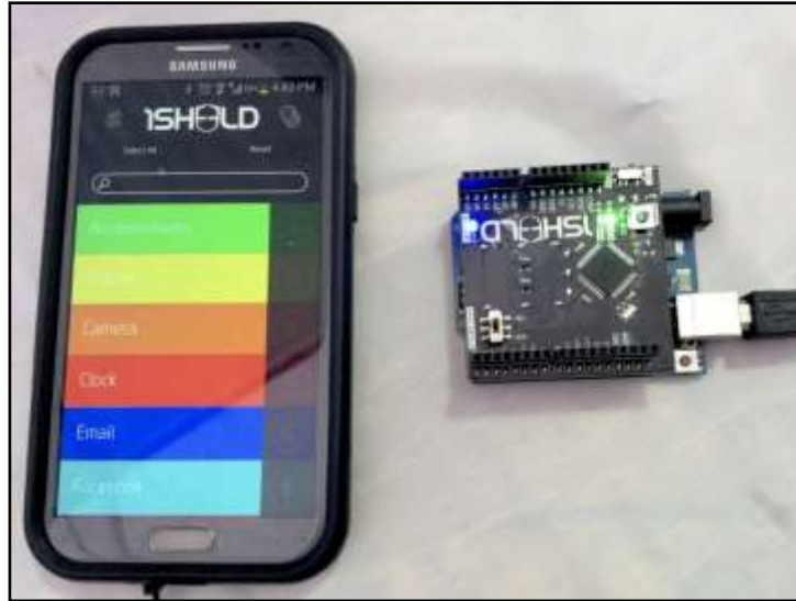
Figure 2. 1Sheeld as a shield for Arduino
